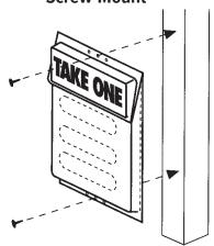
Use the enclosed screws to install Outdoor Literature Holder on any wood post. Make sure to apply the screws through the upper **AND** lower holes as shown.
