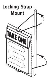
Thread permanent locking straps through the pair of holes located at the top **AND** bottom of the holder, wrap locking straps around pole and thread one end of strap through the open end, then pull tight. **NO TOOLS NEEDED.**
