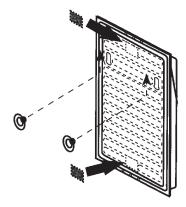
To attach Outdoor Literature Holder to any window, punch out keyhole tabs located on the back of holder and insert suction cups as shown.
